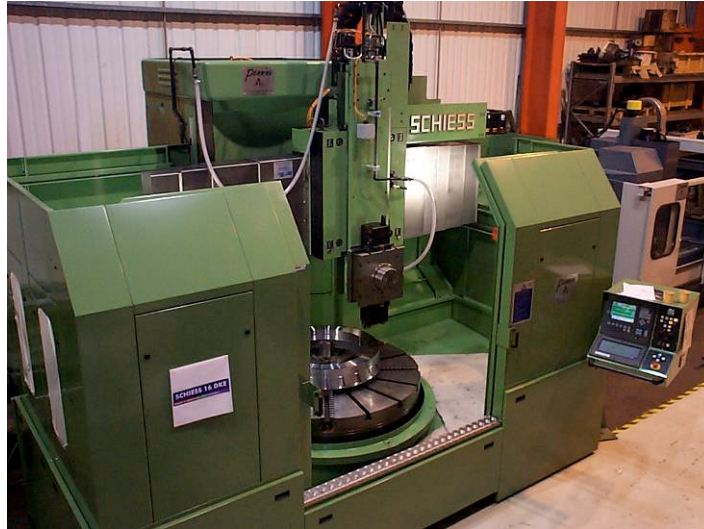
Schiess 14DE , 1250 mm table, elevating rail, CNC Vertical turning and boring machine with 4 station auto turret and Fanuc 21i -T CNC control
